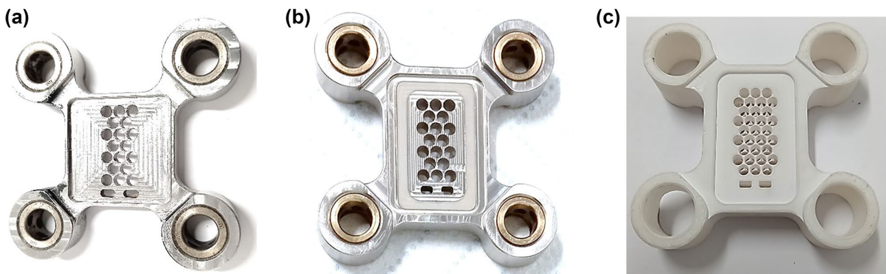
Fig. 17 Three different support configurations tested: steel supports (a), steel supports with PEEK insulation (b), and 3D-printed supports (c)
